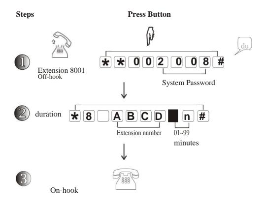
**Description:** Allow to control extension users to do not occupy the conversation and telephone line for long time.
